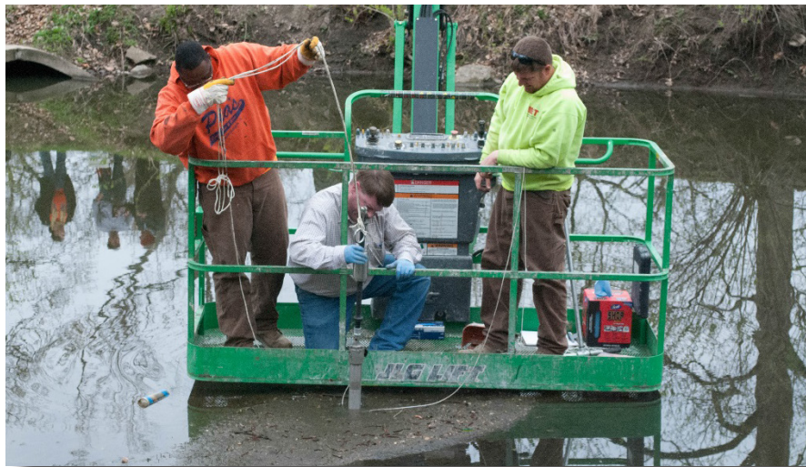
Technicians from Midwest Engineering & Testing taking a core sample from the sediment forebay
