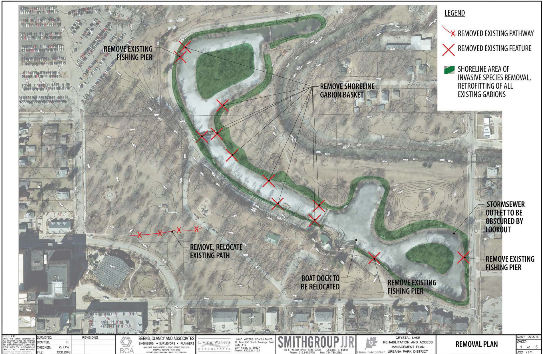
A map showing the current features to be removed during the rehabilitation of the lake, focusing on past shoreline stabilization and outdated fishing piers.
